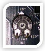
The **DELAY TIME** trimmer enables the user to set the duration (from 20" to 120") after which the acoustic and visual alarm signals are to be shut off (if the flashing light is installed) automatically.
