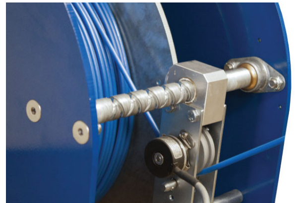
Level wind has been designed to provide a higher degree of cable management
